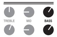
For the most balanced sound and a balance of power between the three rotary tone controls, try to use the TREBLE control in its middle ranges. This scenario produces nearly equal representation of all the frequencies on the tone controls and provides a great neutral starting point for further tweaking.
